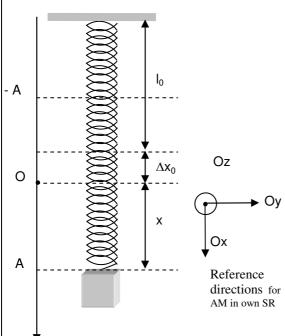
Fig.5. Elastic Pendulum
